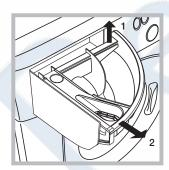
ser by raising it and pulling it out (see figure). Wash it under running water; this operation should be repeated frequently.
